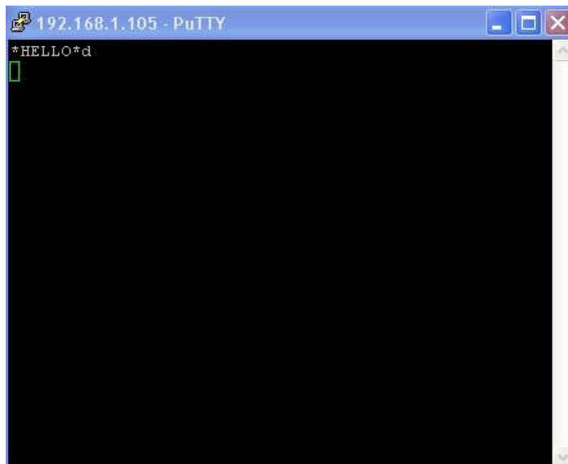
Send ASCII command 'd' ->All relays on
